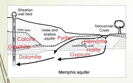
These minerals are potential reactants that traveled through the flow path by the way of the leakage in the confining layer
