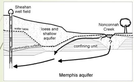
A discontinuity of the impermeable clays in the confining unit result in contamination
