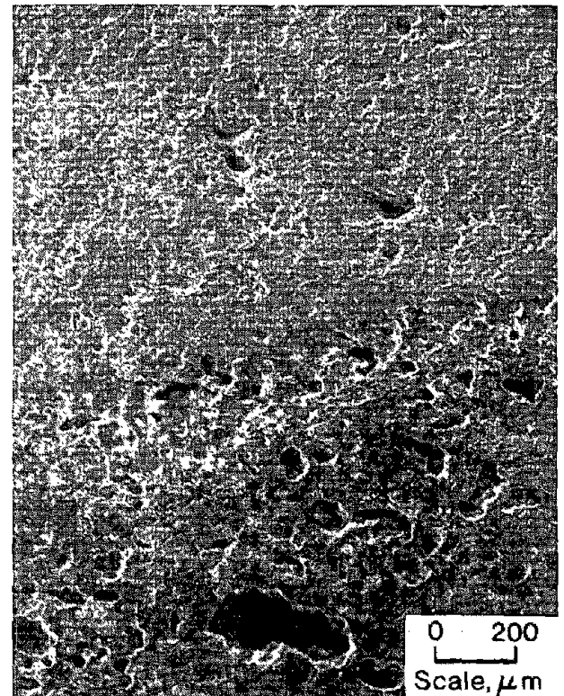
Figure 5.—SEI of Mn ore from Algoma-Zeno deposit (shown in figure 3) showing resulting porous topography after leaching Mn from lower half of mixed pyrolusite-hematite ore.
