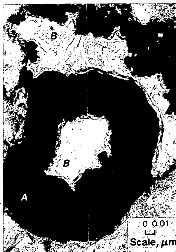
Figure 18.—Photomicrograph of successfully leached chrysocolla encapsulated in goethitic atoll structure (0.16 mm across) (A). Remnants of amorphous silica (clear, with slight relief) (B) can be seen in voids that were once filled with chrysocolla.
