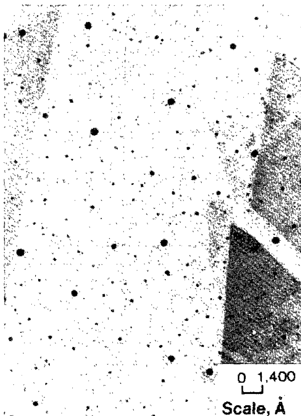
Figure 13.—TEM image of native Cu inclusions in biotite. View is down c-axis of biotite crystal (i.e., perpendicular to cleavage). Image illustrates discoidal shape of inclusions.
