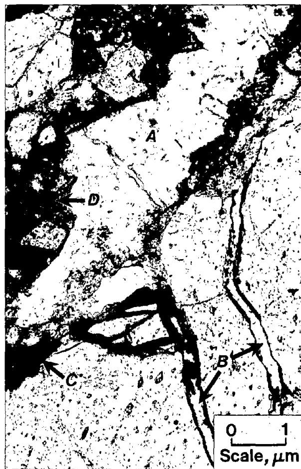
Figure 1.—Photomicrograph of fracture-hosted chrysocolla mineralization from Santa Cruz oxidized porphyry Cu deposit. Mottled yellow chrysocolla vein (A) and 0.14-mm wide blue chrysocolla veins (B) fill 1.4- to 2-mm-wide microbreccia fracture and are associated with quartz fragments (clear), goethite mineralization (dark orange to opaque) (C), and jarosite (mottled brown) (D).
